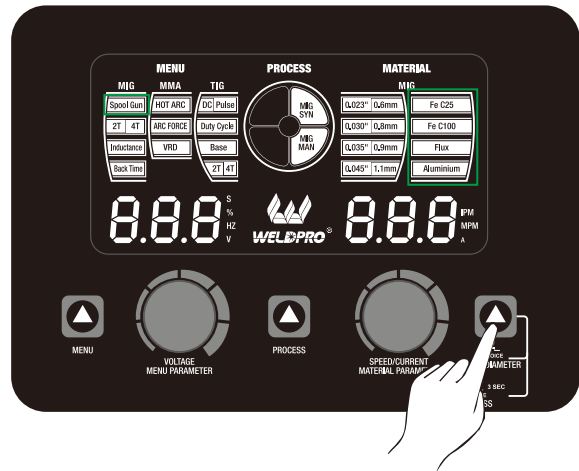
Step 4. Press and hold the WIRE DIAMETER button for 3 seconds to choose MIG shielding gas, FCAW, or Aluminum (spool gun). Gas or FCAW selection will affect voltage and wire speed settings in MIG SYN mode. Aluminum must be selected in MIG SYN or MIG MAN mode to use the spool gun.
